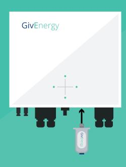
IMPORTANT! Please ensure the dongle is screwed into the bottom of the inverter on both sides.
